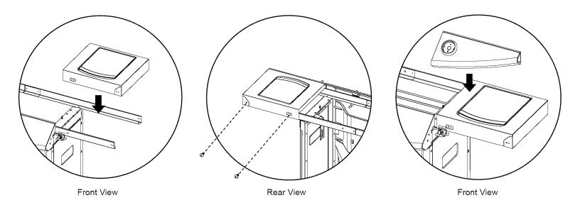
22. Attach side burner assemblies using shelf mounting procedures as previously described. (Steps 14 & 15)
